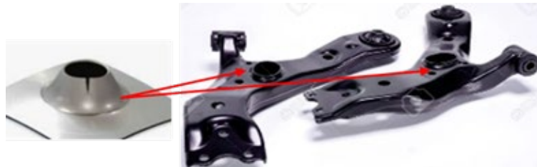
Fig.2 Samples After Hole-Expansion Test and Typical Flanged Auto-Components (Ref: 5~6.)
